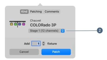
2 If the fixture has different operation modes (or "personalities"), select a mode from the pop-up menu below the fixture name. Be sure to select the same mode as on the fixture, or Lightkey will not be able to control the fixture! If no menu is shown then the fixture has no modes.
